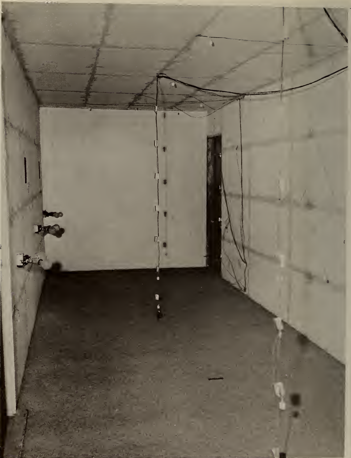
Figure 12. Interior View of Corridor. Fire Room at Right Rear. Thermocouples on Walls in Center of Corridor, Radiometers in Floor.
