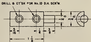
LATCH RETAINER 1 REQ. ALUM.
