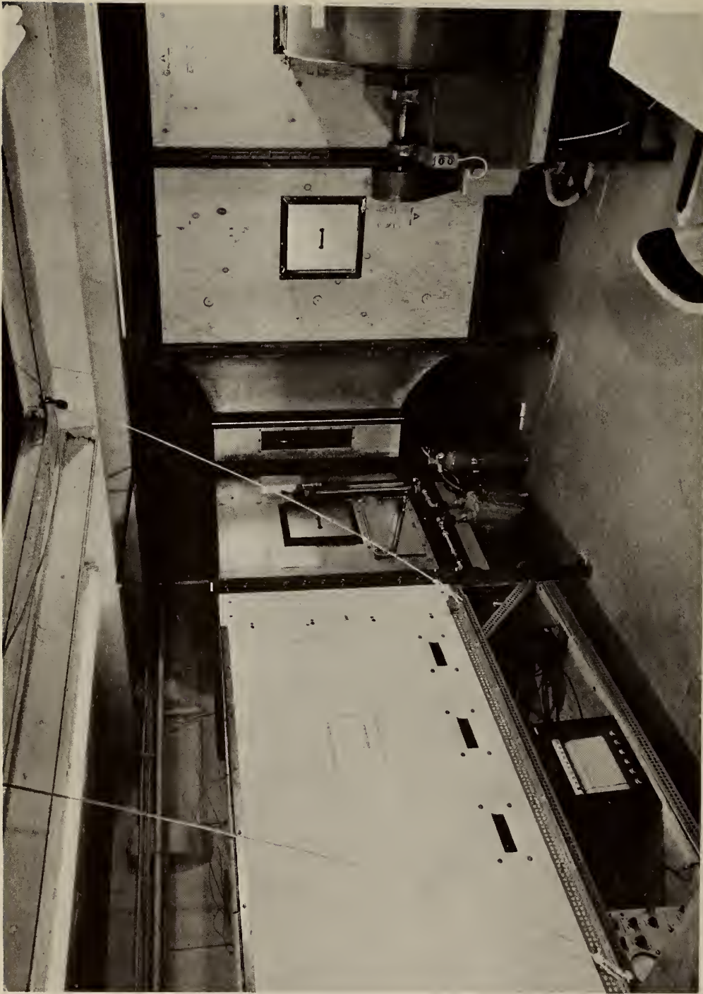
Figure 16. Carpet Flammability Duct Apparatus. Air Supply System at Right, Combustion Chamber at Left.
