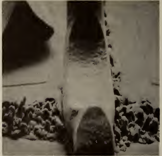
a. Small bond deformation ( \sim 1.2 times wire diameter). Magnification \sim 585 X.
