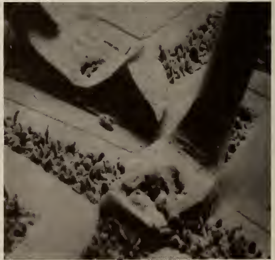
c. Large bond deformation ( \sim 2.2 times wire diameter as determined from head-on SEM photomicrograph). Magnification \sim 230 X.
