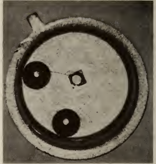
b. Photomicrograph of TO-5 header with 40-mil (1.02-mm) square diode chip bonded over dimple. Magnification \sim 6.4 \times .
