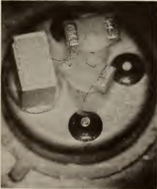
Figure 26. Photomicrograph of typical R-C plug-in network assembled on a TO-5 header. (Magnification \approx 8.4 \times ).
