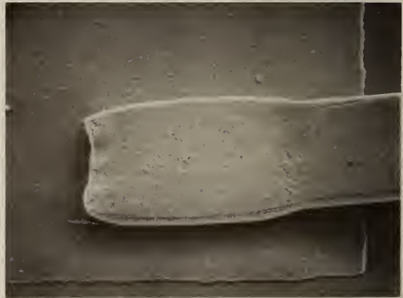
b. Second bond. Magnification \sim 470 \times .
