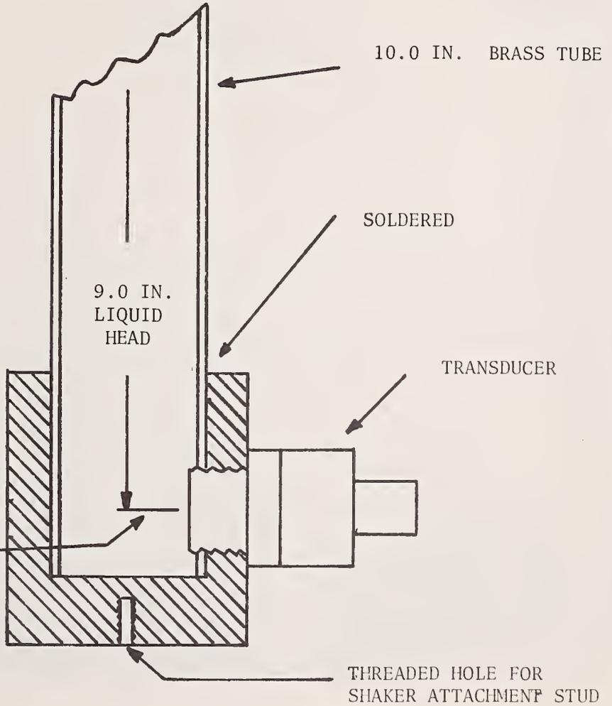
SINUSOIDAL PRESSURE CALIBRATOR MOUNTED
