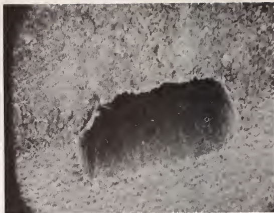
Figure 9. SEM photomicrograph of a rectangular wire-feed hole in an ultrasonic bonding tool. (There is a slight build up of aluminum in the upper left corner of the hole. Magnification: about 750 X.)
