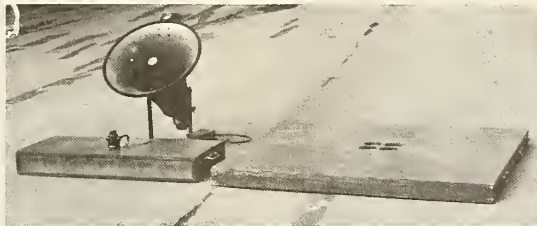
Figure 3. Sound sources used for the measurement of the sound insulation of facades.
