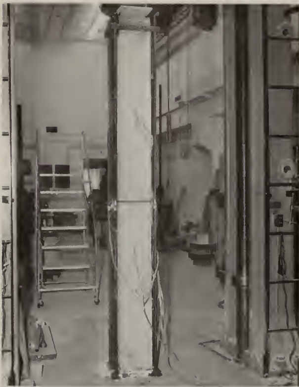
FIGURE 17. Test specimen with grouted dowel.
