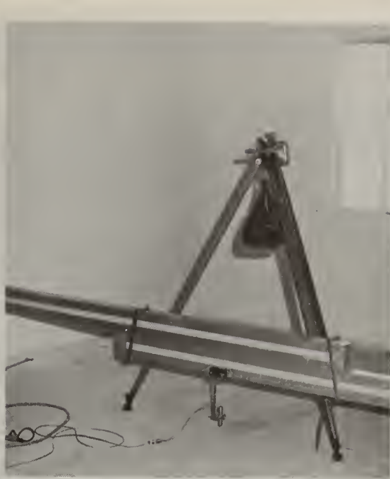
FIGURE 4. Apparatus for measurement of transient floor vibrations.
