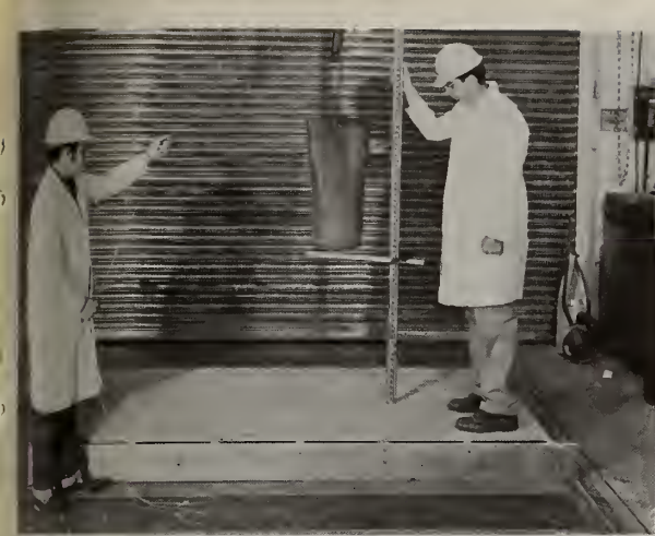
FIGURE 3. Apparatus for impact tests on floors.
