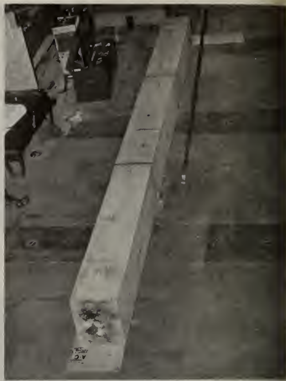
FIGURE 18. Shear-test specimen before grouting.
