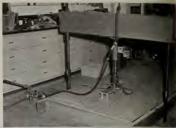
FIGURE 6. Apparatus for concentrated load test on floors.
