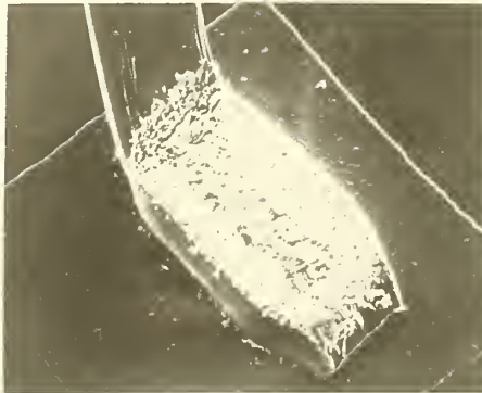
Figure 7. SEM photomicrograph of overbonded ribbon-wire first bond. (Magnification 400 x)
