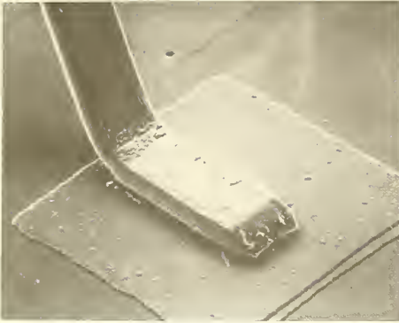
Figure 5. SEM photomicrograph of typical ribbon-wire first bond. (Magnification 350 x)
