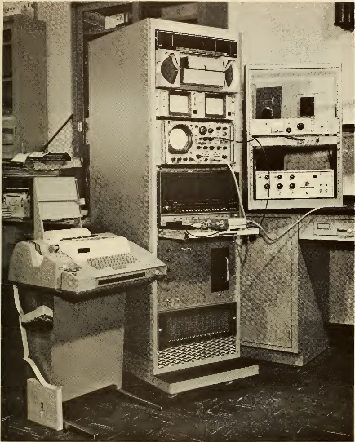
Figure 5-2. Photograph of Time Domain Automatic Network Analyzer (TDANA).
