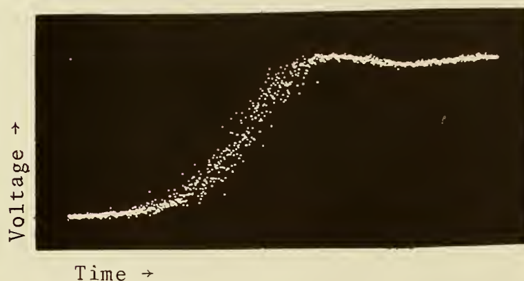
Figure 9-4. 1024-Point Single-Waveform Representation of a Tunnel Diode Pulse Acquired on the TDANA. Oscilloscope Settings Were 50 mV/cm and 10 ps/cm.
