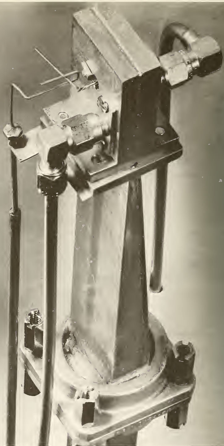
Figure 4. The broadband microwave (X-band) SQUID. The mechanism for adjusting the point contact via a push rod can be clearly seen.
