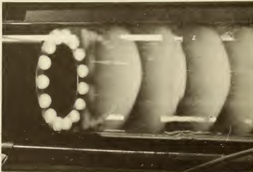
Figure 2 b. Ring anode and resulting stable plasma configuration.
