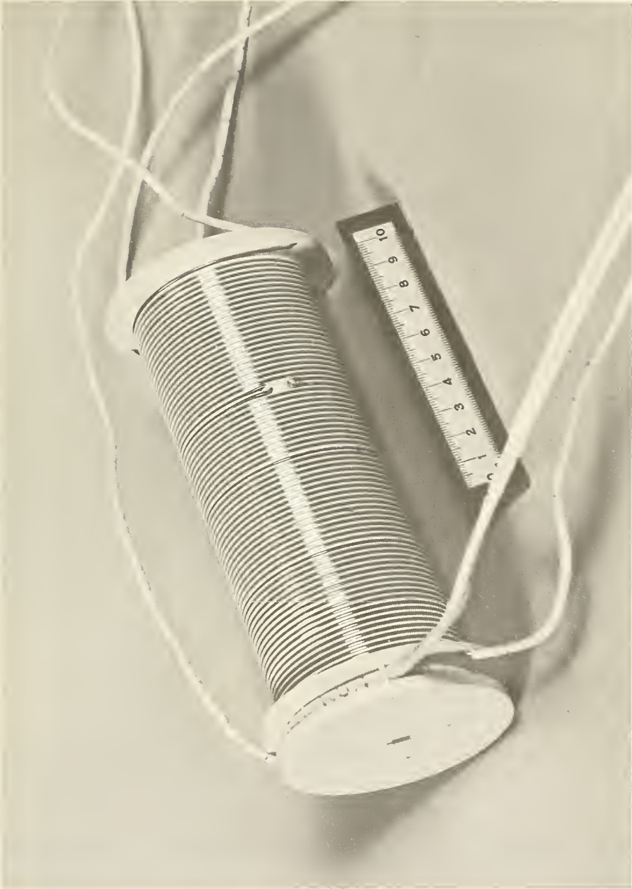
Figure 3.7. Photograph of the Assembled Boron Nitride Heat Distributor.
