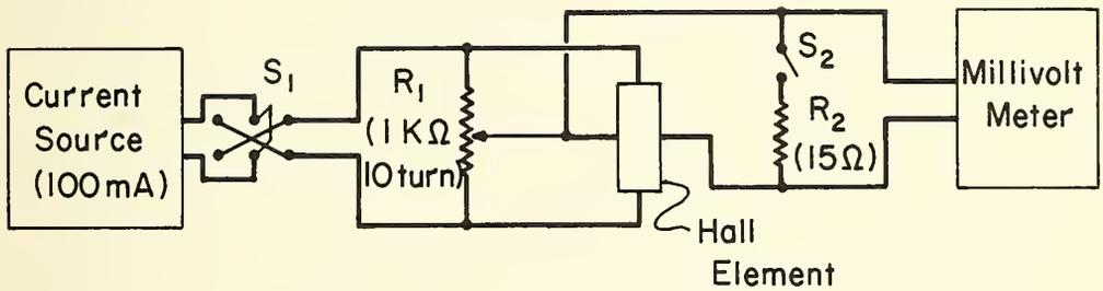
Figure 2. Circuit diagram for resistive voltage offset zero.
