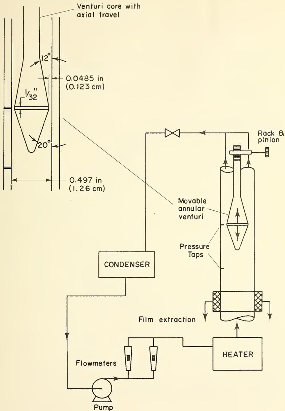
Figure 1. Flow circuit of the steam-water loop
