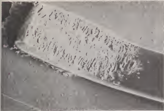
Figure 8. SEM photomicrograph of a well made ribbon wire bond. (Magnification 530 X)
