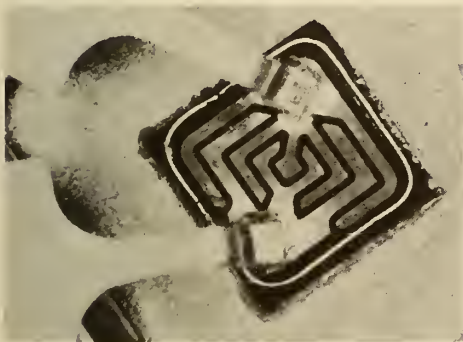
c) 2N3878 transistor chip. These transistors had the aluminum metallization covered by a layer of aluminum oxide.
