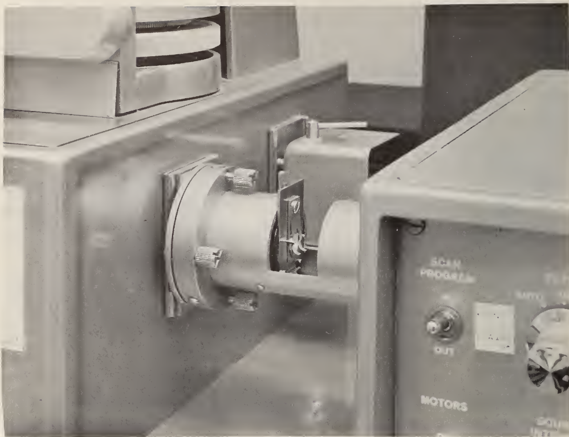
Figure 20. Infrared beam condenser (4X) containing a 1 mm KBr sample pellet.
