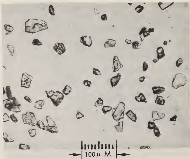
Figure 2. Photomicrograph of 30-60 \mu m silica gel used in resistance tubes.
