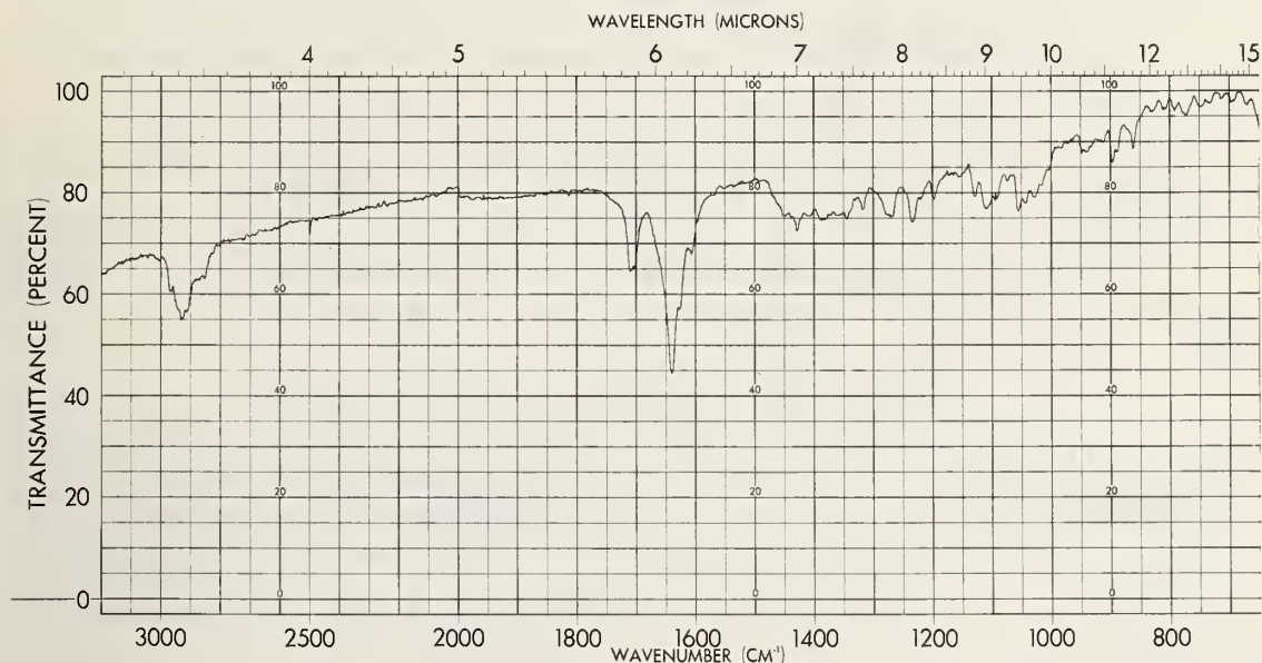
Figure 14. Infrared spectrum of 10 \mu g of cortisol obtained by concentration.
