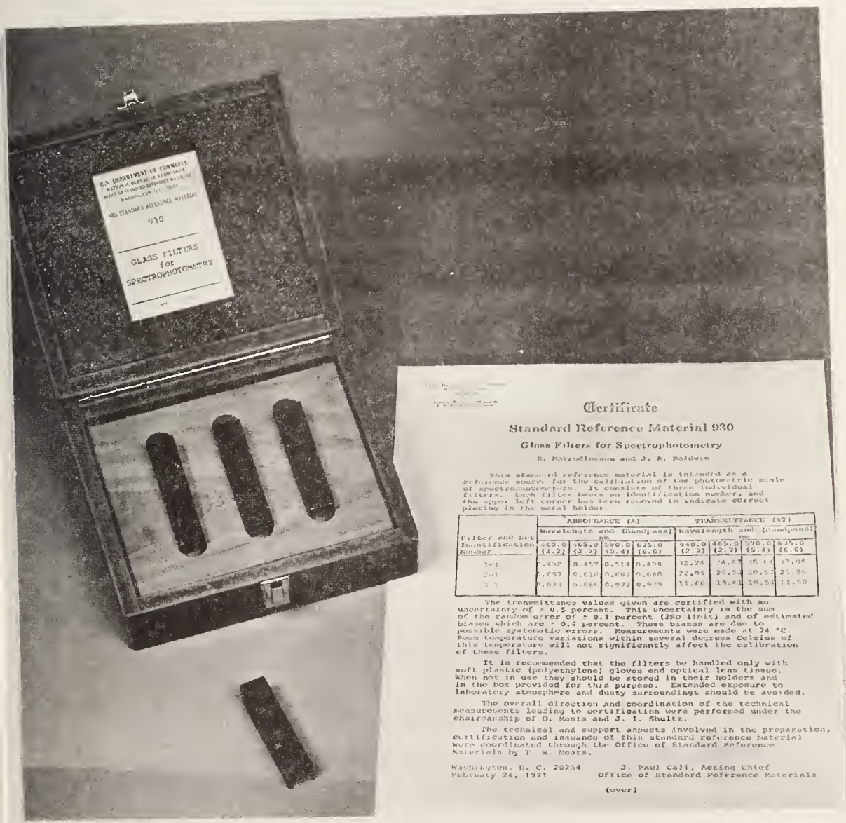
Figure 1. Set of three glass filters with the corresponding provisional certificate constituting SRM-930.
