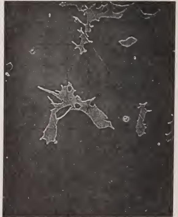
Figure 13. Electromagnetic translation of the field of view. Target current images of a two-phase nickel-aluminum alloy. One large division equal to  $66 \mu\text{m}$  (150 X).
