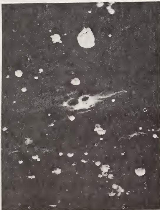
Figure 21. Absorbed electron scanning image of fly ash particles mounted in collodion. Magnification: 25  $\mu\text{m}/\text{cm}$ .
