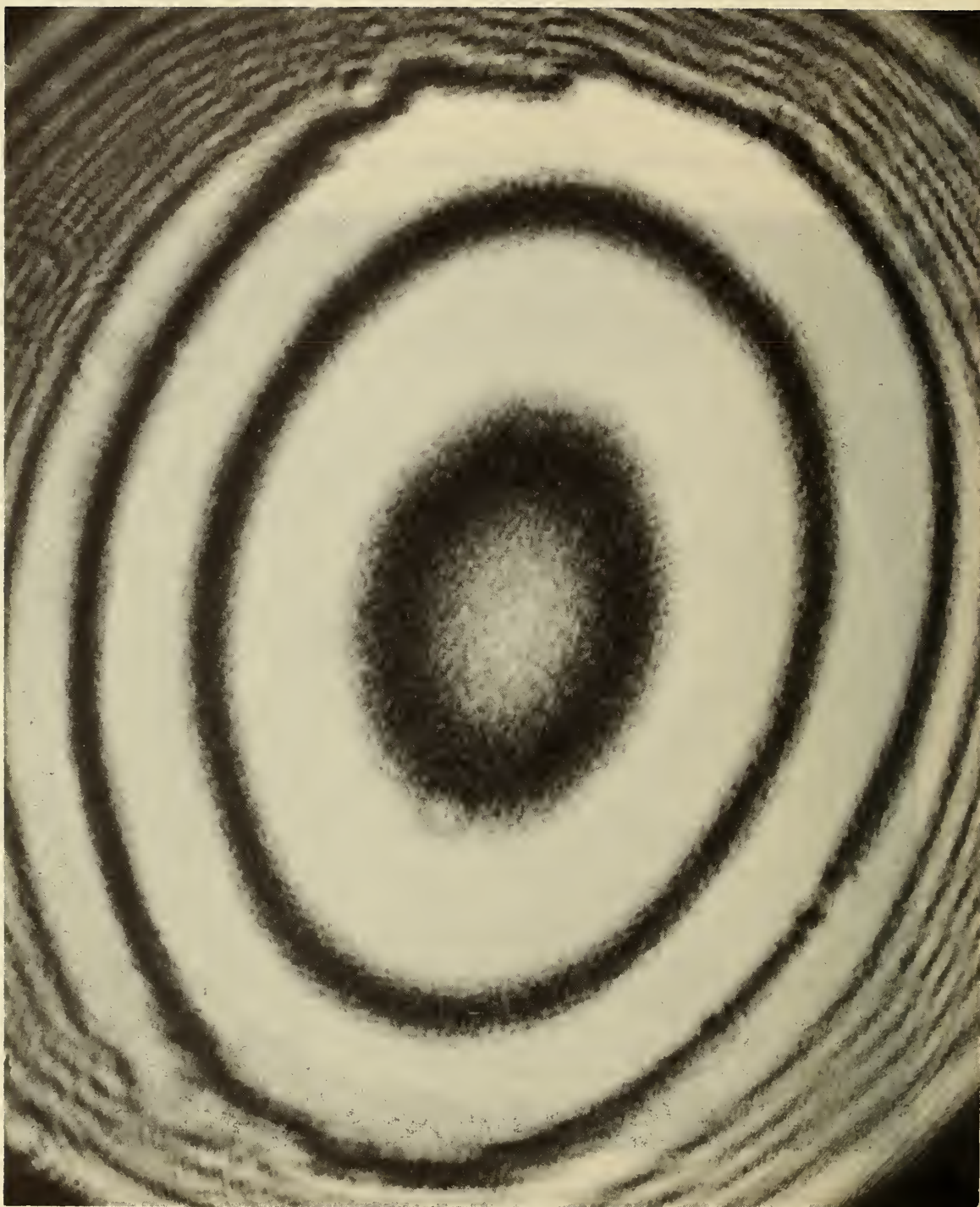
Fig. 2(a) Twyman-Green interferogram of ten plate tent polarizer in oscillator system. Three elliptical fringes are shown which indicate that the polarizer is acting as a weak positive lens.
