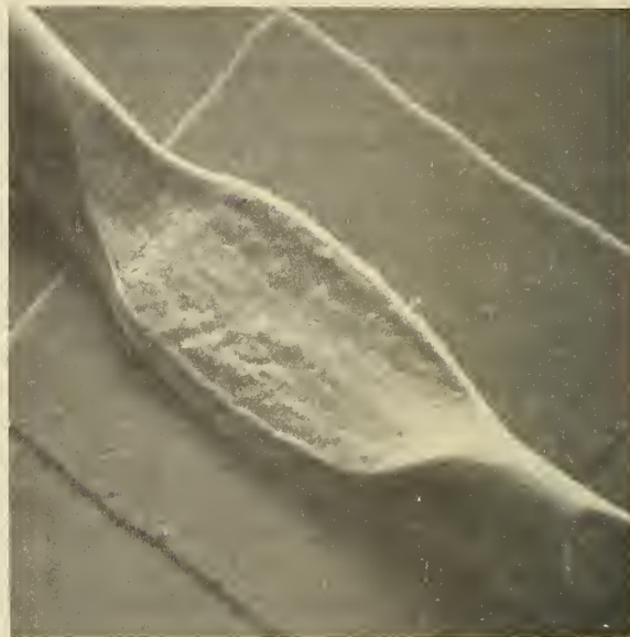
c: Amplitude: \sim 25 \mu\text{m} ; Frequency: 20 Hz; Magnification: 500 X.
