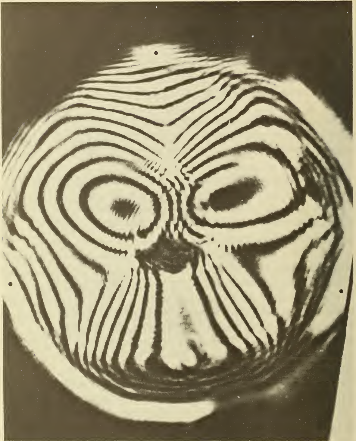
Figure 1. Twyman-Green interferogram of YAG boule.
