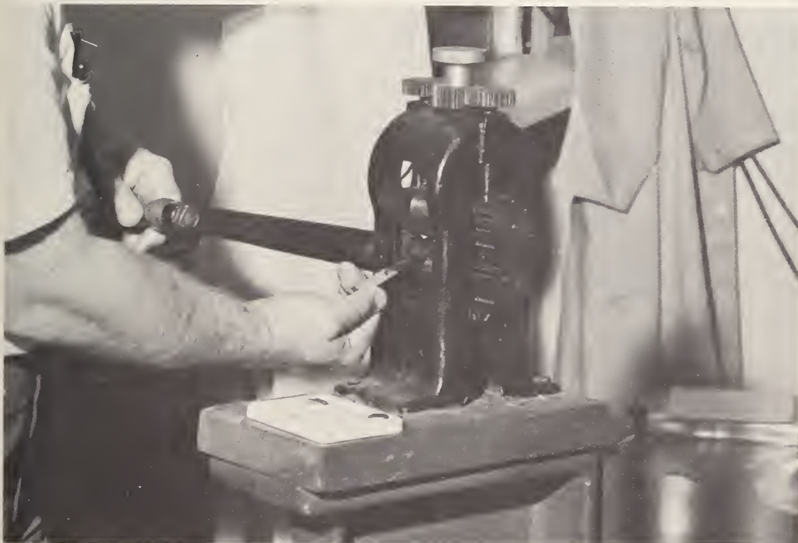
Figure 17. Lead alloy ingot being rolled into a thin foil.
