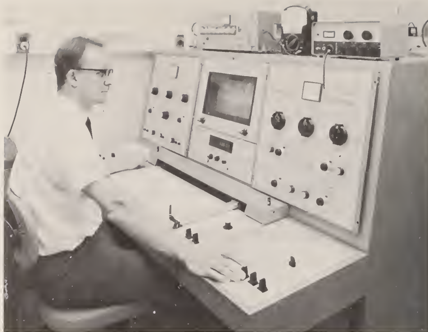
Figure 4. Adjustment of the strength of the magnetic field, at the console of a nuclear magnetic resonance spectrometer.
