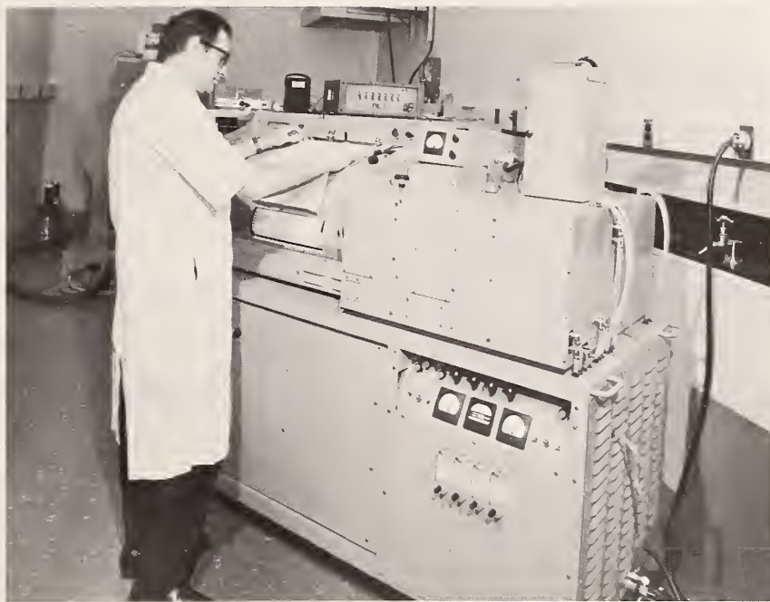
Figure 2. Recording an optical rotatory dispersion spectrum.
