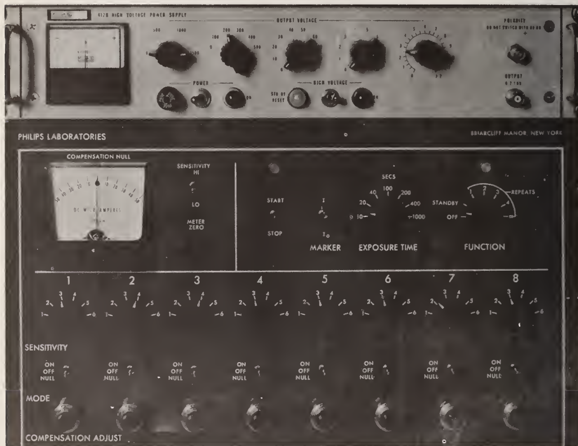
Figure 37b. Front panel of the electronic system shown in 37a. From bottom to top -- dark current compensation, channel sensitivity selectors, mode of operation switches, power supply for photomultiplier tubes.
