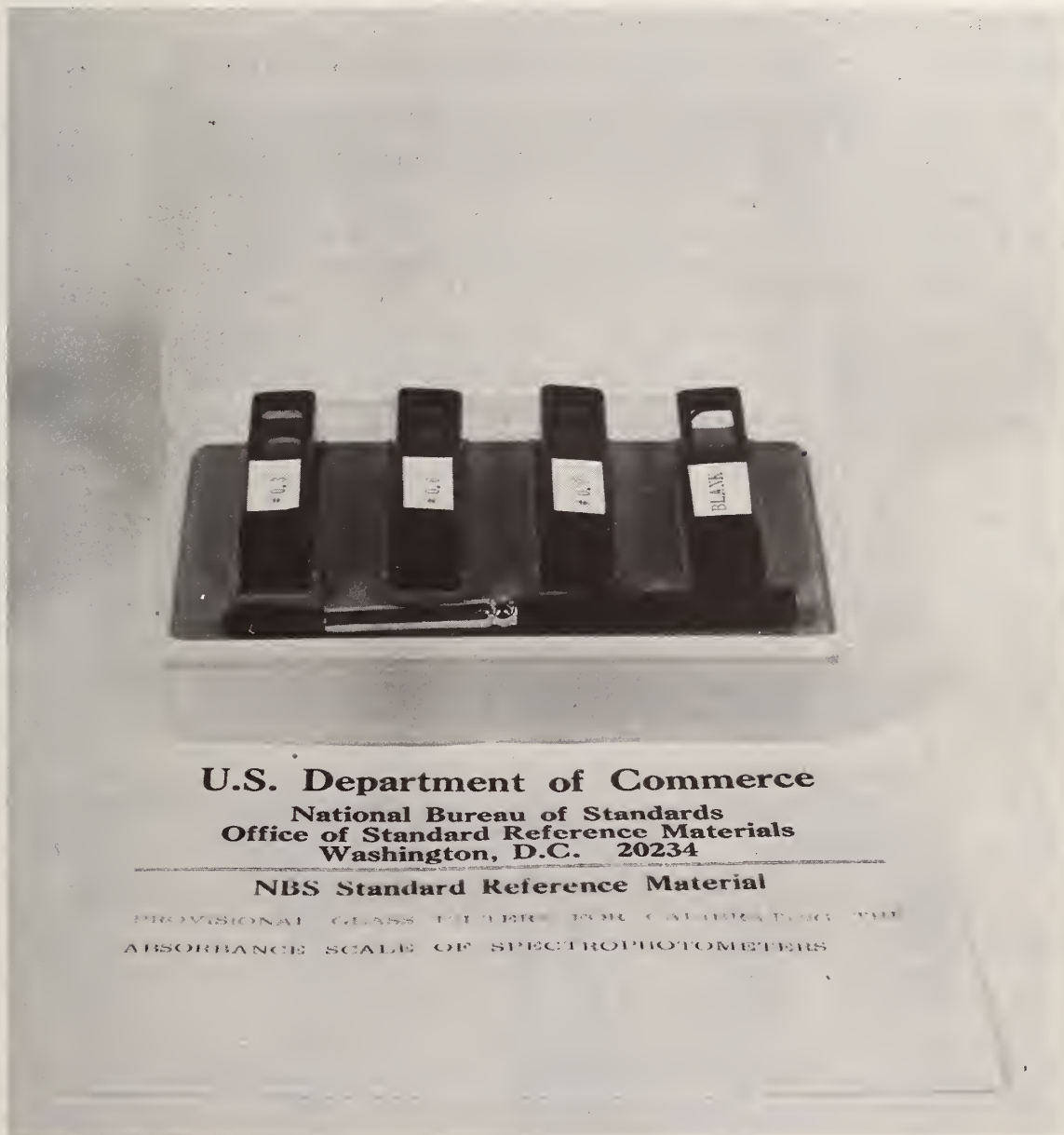
Figure 4. Presentation of a set of provisional filters made from evaporated metal on quartz.
