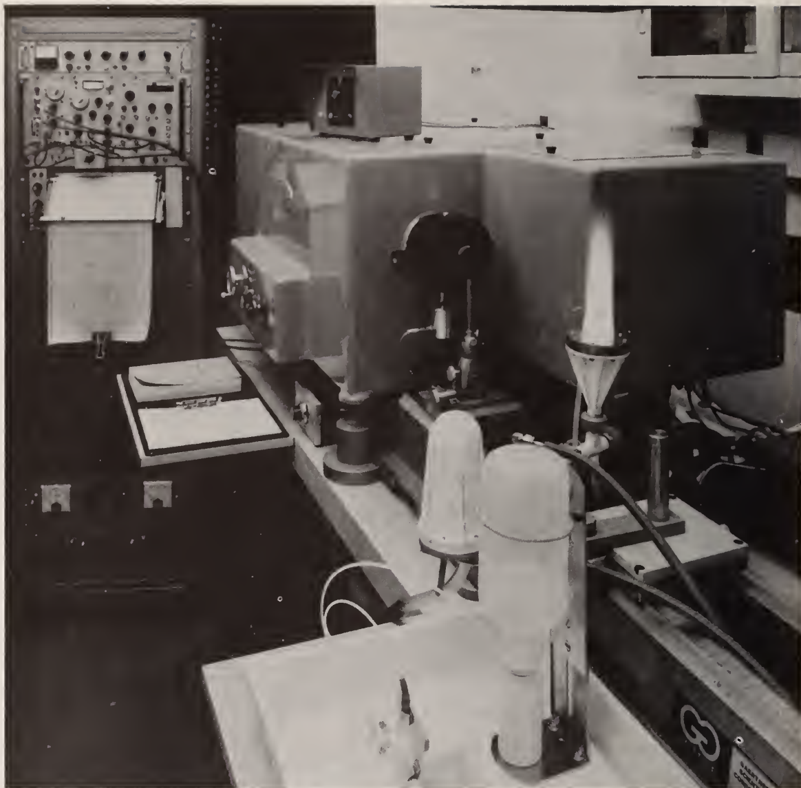
Figure 32. Flame spectrometer. Left - console with the electronic measurement system for the scanning mode system, and power supply for the hollow cathode. Middle - one meter spectrometer and sprayer and burner unit producing a premixed air-acetylene flame. The pneumatic sprayer is supplied with the analytical solution through a two way Teflon stopcock. Right - water pressure gauge for monitoring the pressure in the spraying vessel and burner unit.
