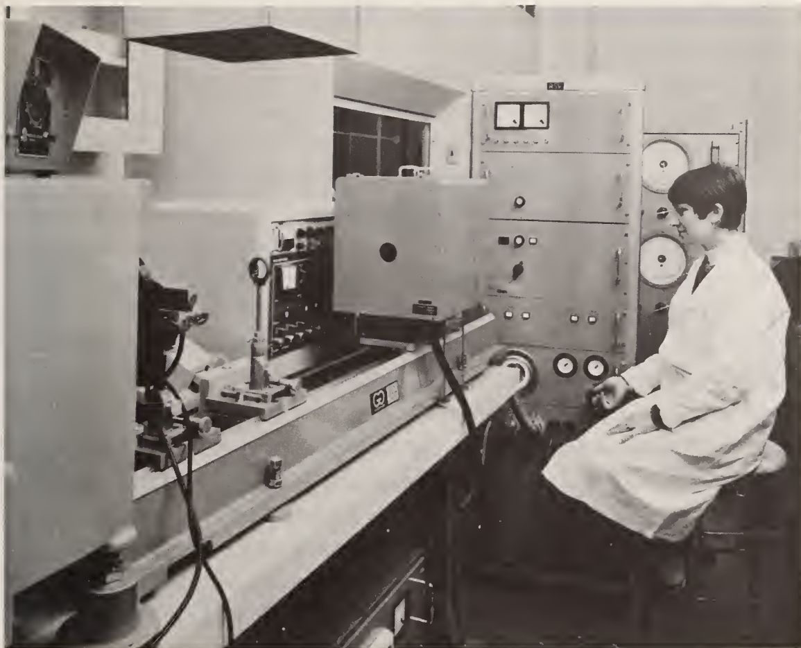
Figure 40. Hollow cathode discharge unit after Grimm. The hollow cathode is located in the enclosure placed on the optical bench. The power supply and various controls are located in the console at the extremity of the optical bench.
