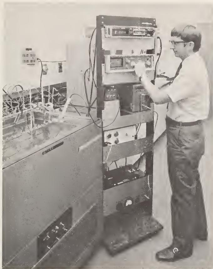
Figure 7. Equipment for measurement of ion-selective electrode cell emf.
