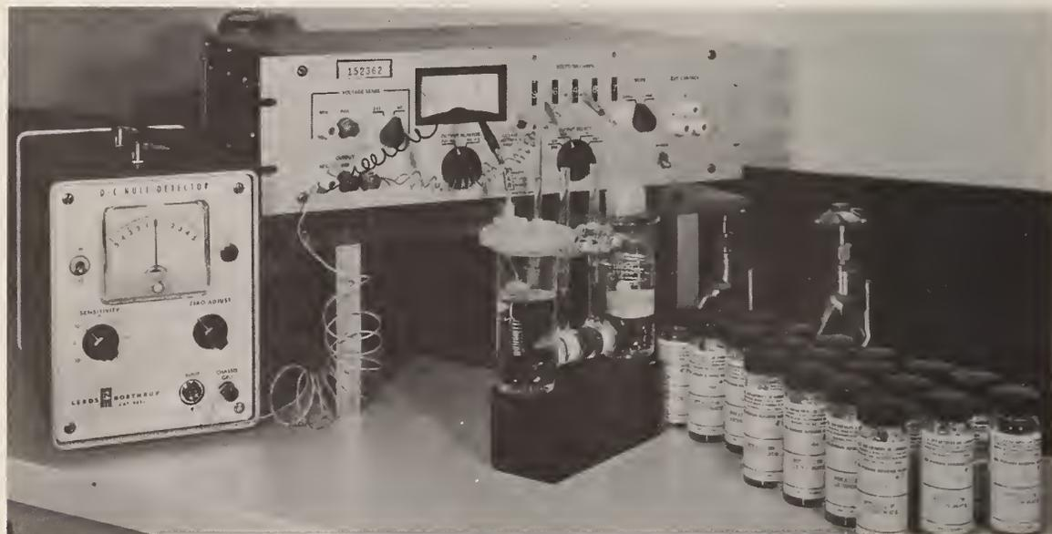
Figure 11. Potassium dichromate samples and some of the coulometric equipment used in standardizing this oxidant.
