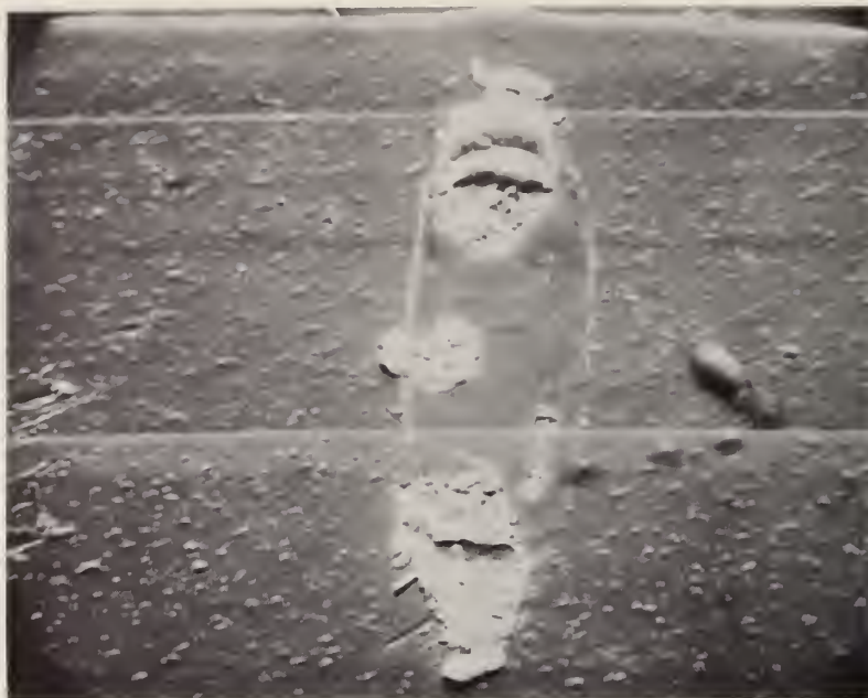
Fig. 18 SEM photomicrograph (800 X) of bond adhesion (lift-off) pattern for a strong first bond.
