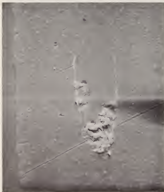
Fig. 19 SEM photomicrographs (600 X) of bond adhesion (lift-off) patterns for two second bonds made consecutively at identical time and power settings.
