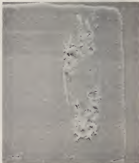
Fig. 19 SEM photomicrographs (600 X) of bond adhesion (lift-off) patterns for two second bonds made consecutively at identical time and power settings.
