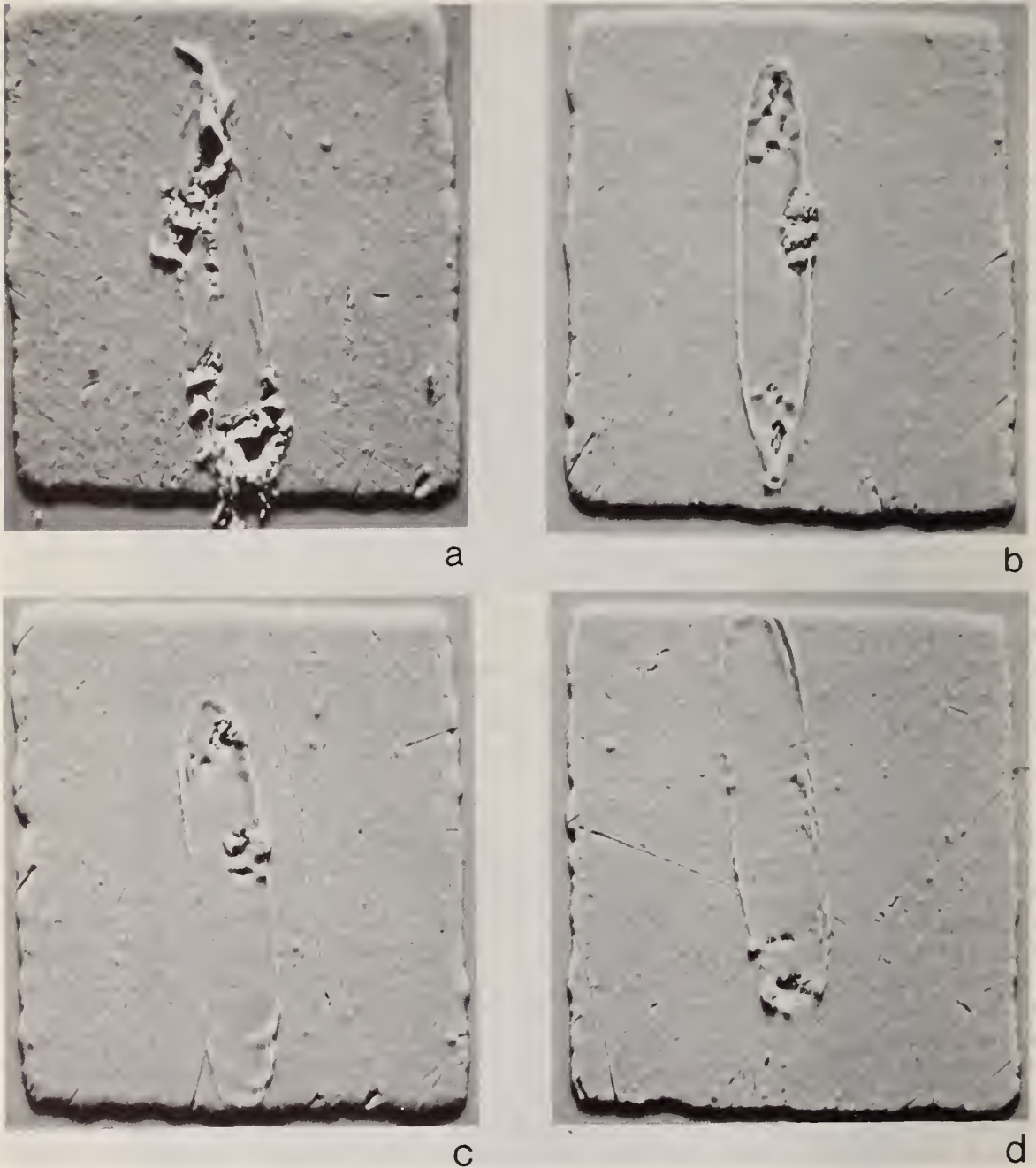
Fig. 17 SEM photomicrographs (460 x) of bond adhesion (lift-off) patterns for first bonds made at different time settings and constant power setting. The time is longest for case a and is decreased to the shortest value for case d. Settings used in case a result in a bond which will adhere to the pad; the shorter time settings do not produce an adherent bond. Note that the scratches on the bonding pads (which result from a cleaning process no longer in use) are polished out by the ultrasonic motion of the compressed wire even before appreciable bonding occurs. Note also the apparent movement during bonding exhibited in case d. This is thought to result from mechanical vibration in the bonding machine.
