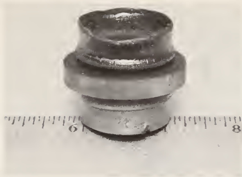
Figure 32. Penning ion source: side view of burned aluminum anode
