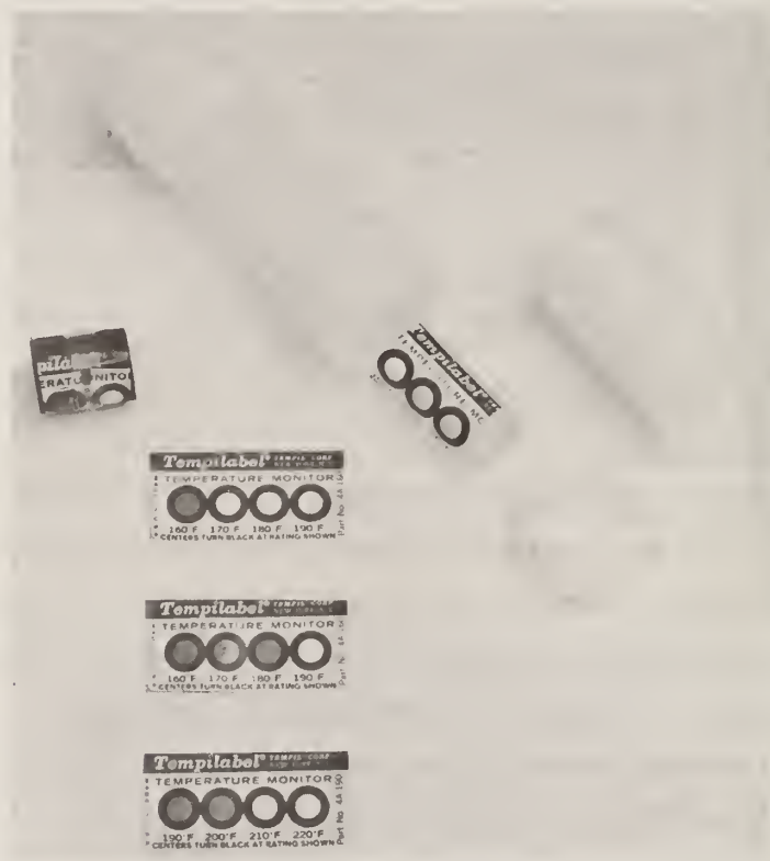
Figure 9. Temperature sensing labels, NBSR "rabbit" and quartz blocks used for temperature measurement
