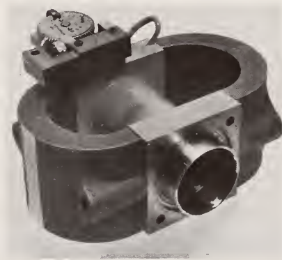
Figure 34. Penning ion source: assembled, showing mechanical gas lead, and U magnets
