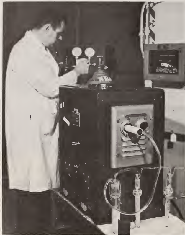
Figure 41. Resistance furnace and collecting train for carbon determination
