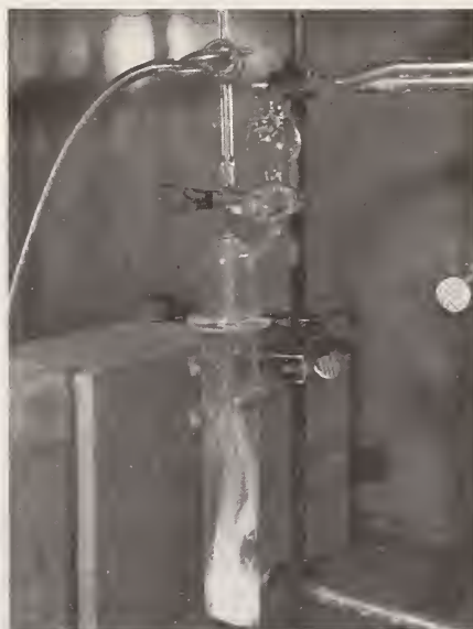
Figure 44. Combustion of sodium for carbon determination
