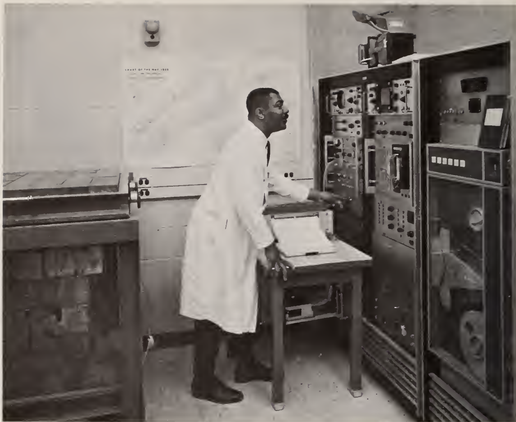
Figure 14. Counting room showing shield for Ge(Li) detector and 4096-channel analyzer
