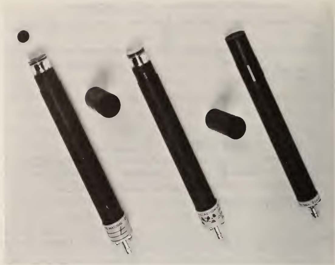
Figure 12. Sample mounting for one phototube technique
