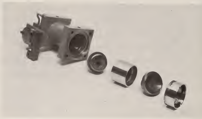
Figure 30. Penning ion source: disassembled
