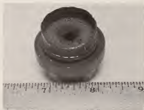
Figure 31. Penning ion source: inside view of burned aluminum anode
