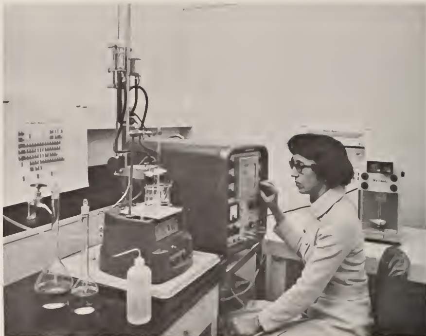
Figure 3. Apparatus used for EDTA determination.
