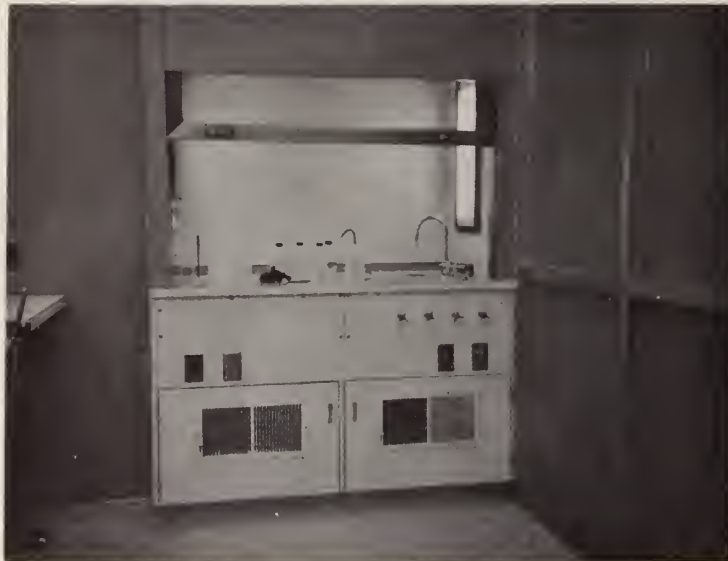
Figure 23. Vertical laminar flow fume hood in Class 100 area. The baffle wall separating the two areas is on the right.
