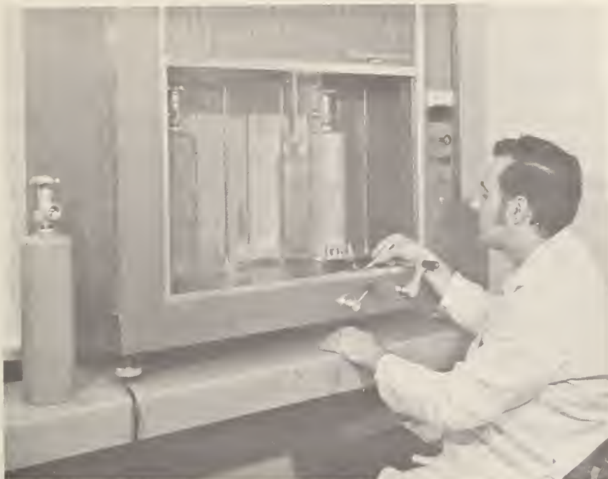
Figure 1. Preparation of standard gas mixtures by weighing.
