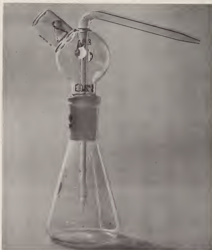
Figure 15. Apparatus for dissolution extraction of iron in high purity gold.
