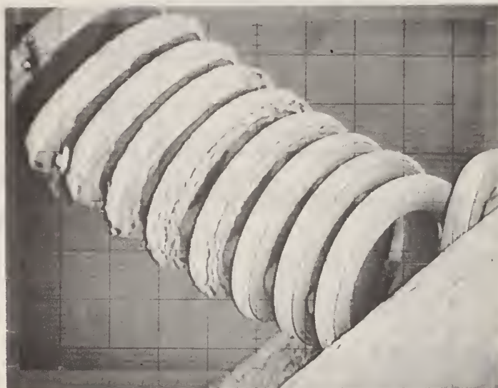
Figure 16. Scanning electron micrograph of a partially recrystallized lamp filament. 20 keV, 10^{-8} A. Mixed target signal. Magnification: 200X.
