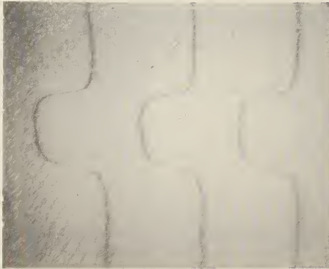
Fig. 3 Interference pattern of a 1.7 \mu\text{m} -thick aluminum stripe as observed on multiple-beam interferometer.
