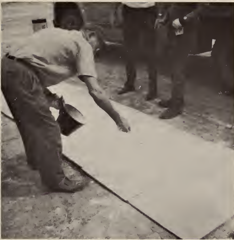
FIGURE 1. Coating of insulation boards with lime dust to prevent adhering of field samples.
