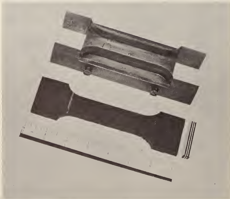
FIGURE 4. Cutting die, built-up roofing specimen and cross section of membrane.
