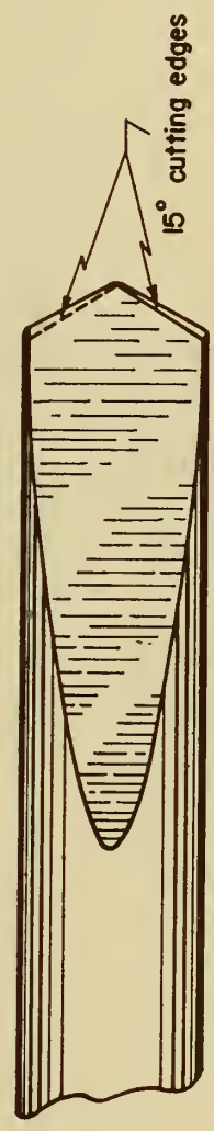
Fig. 2. Tungsten carbide tool for drilling the longitudinal hole in the tungsten tube furnace.
