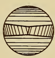
Fig. 2. Tungsten carbide tool for drilling the longitudinal hole in the tungsten tube furnace.
