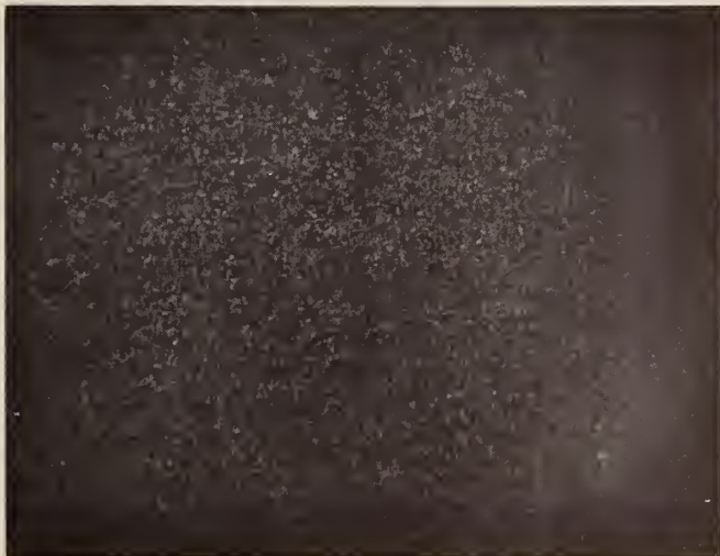
Figure III-1(c). Electron-probe scan of annealed (\text{Cu}_{0.90}\text{Ni}_{0.10})_{0.92}\text{Fe}_{0.08} using \text{FeK}\alpha X-ray.
