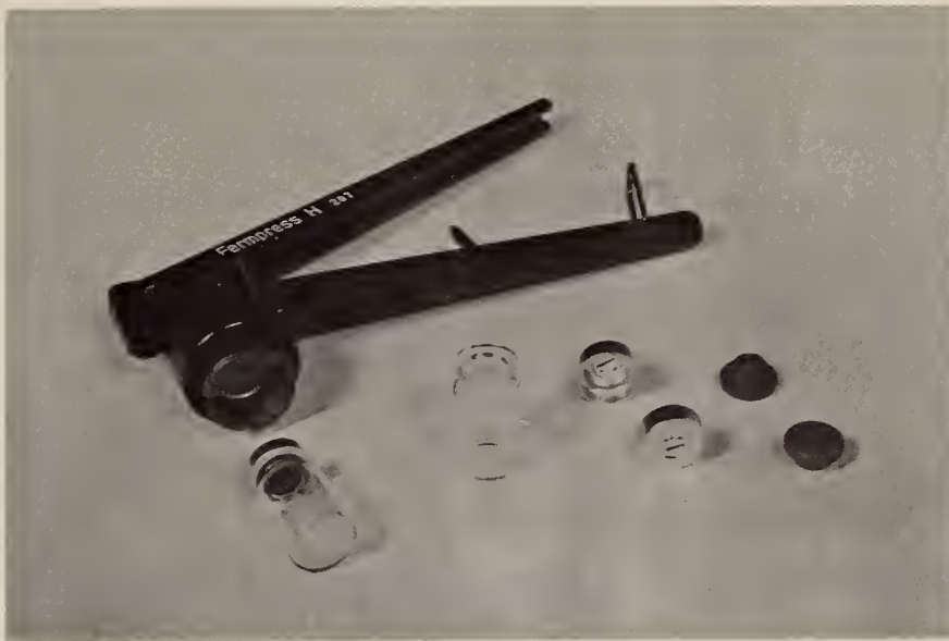
Figure 19. Photograph of rubber septum vials that have been used to assist silylation gas chromatography.
