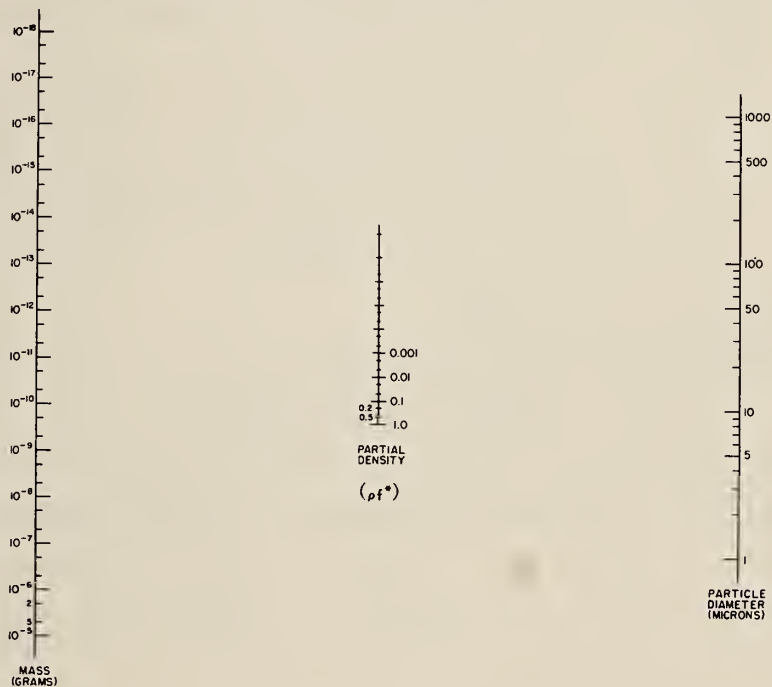
Figure 14. Nomogram for determining mass of counterion as a function of particle size and of specific counterion density (grams/millimeter).
