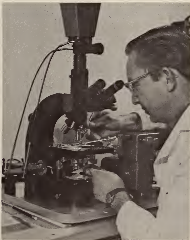
Figure 12. Microscope and micromanipulator are used in the processes of measurement of individual microstandard beads, and for transpositioning to the apparatus requiring calibration.
