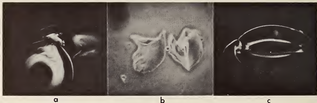
Figure 3. Solvent stressed ion exchange bead (a) disgorging its interior during sulfonation, (b) after disgorgement and (c) a piece of the expelled interior.
