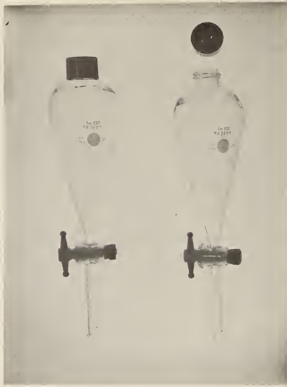
Figure 15. Separatory funnels modified with screw-top closures.
