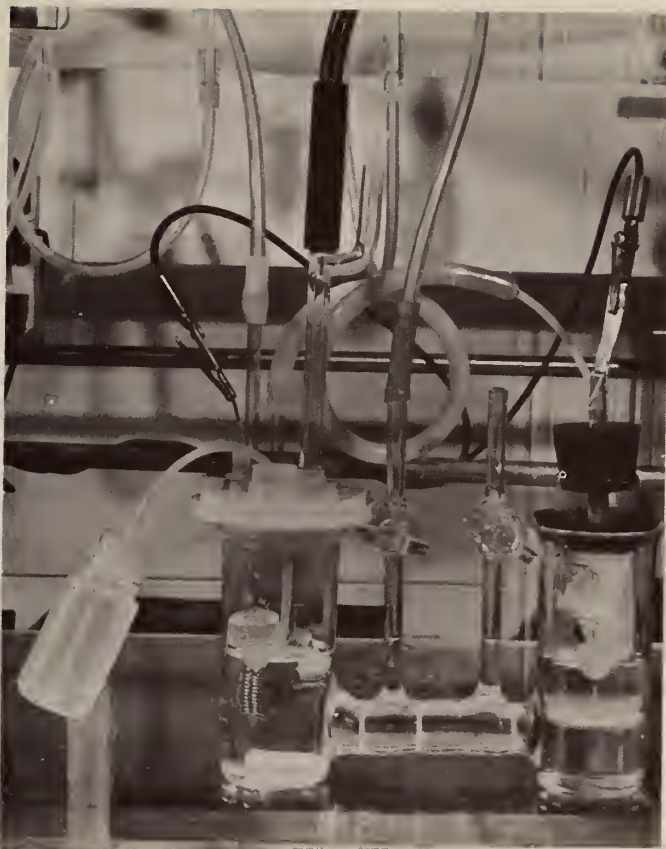
Figure 8. Coulometric titration cell for precise acidimetry.
