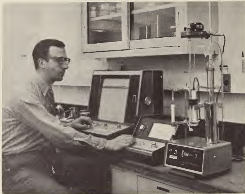
Figure 14. Apparatus for fluoride determination by linear null-point potentiometry.
