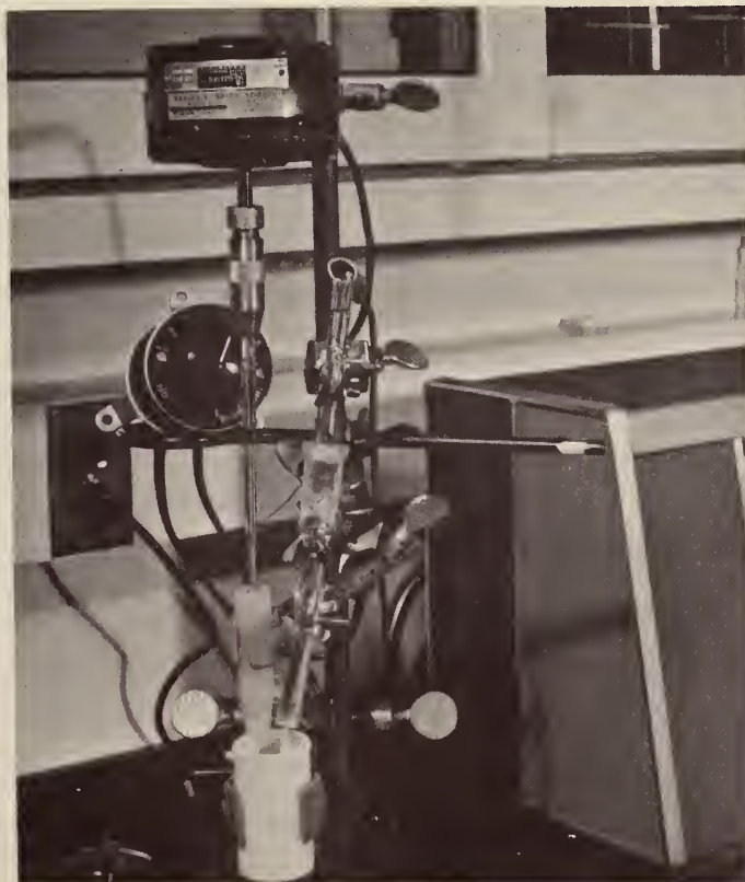
Figure 16. Fluoride generation cell.
