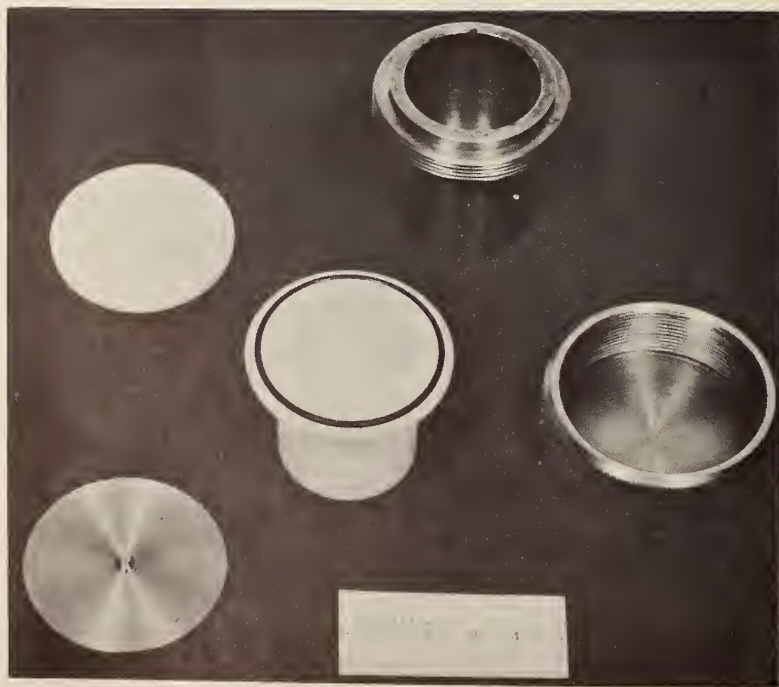
Figure 17. Teflon-lined apparatus for the dissolution of refractory nitrides.
