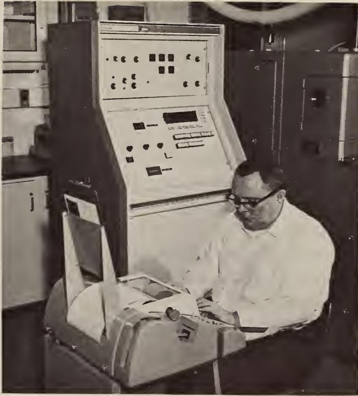
Figure 2. Digital readout for emission spectrometer. (The large console contains the integrating capacitors and electronics for dark-current and background correction and digitizing. Data are printed on the teletypewriter).
