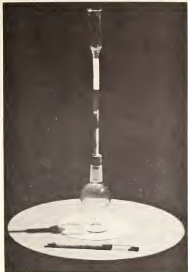
Figure 11. Activated alumina provides an excellent trap for acid and polar impurities in organic solvents. The intensely colored impurities that remain in 99.7% pure material become obvious when a small liquid sample is passed through the tube.
