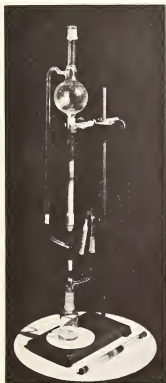
Figure 12. Chromatograph column for removing contaminants from nitrobenzene. Colored zones on activated alumina (neutral) are visible in the extra column section at the base of the stand in the photo. This apparatus is the same as that in figure 11, but on a larger scale and therefore useful for preparative work.
