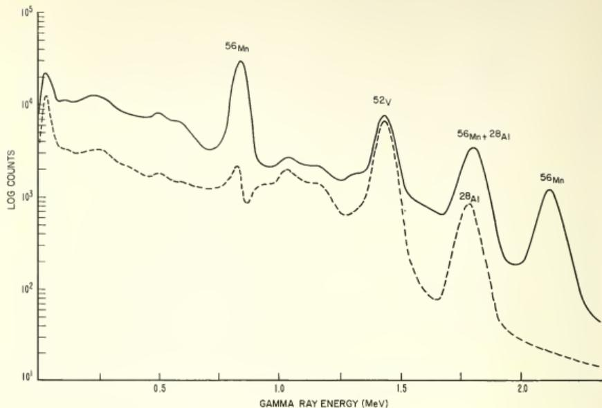
Figure 14. Gamma-ray spectrum illustrating removal of a long-lived contaminant by subtraction.
