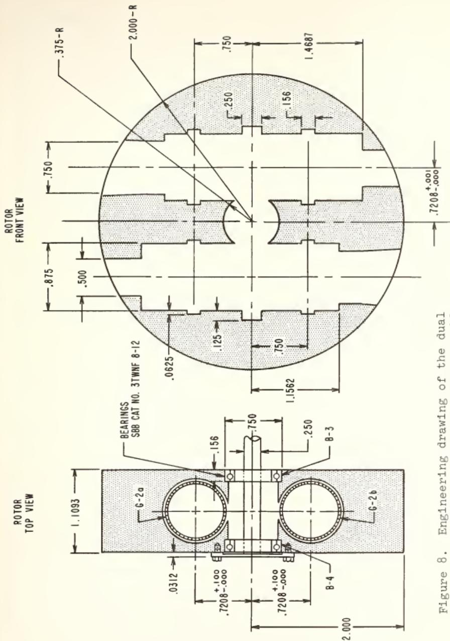
Figure 8. Engineering drawing of the dual sample biaxial rotating assembly.
