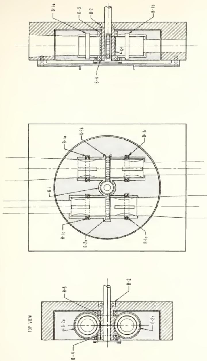
Figure 6. Assembly drawing of the dual sample biaxial rotating assembly.
