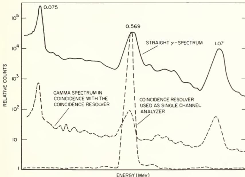
Figure 16. Gamma spectra of  $\text{Bi}^{207}$  and each of the two coincidence spectra.
