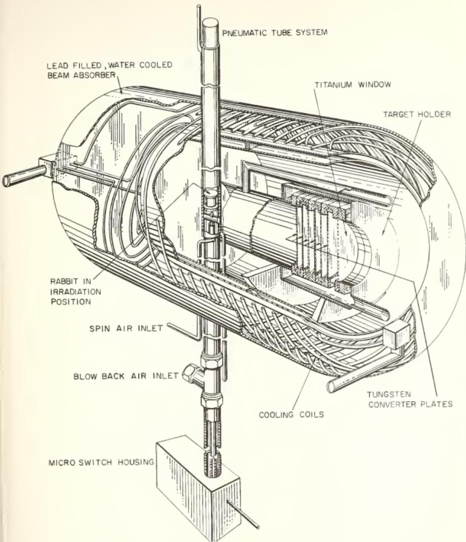
Figure 17. Cutaway view of the target, rabbit terminal, and beam dump as it appears before the beam.
