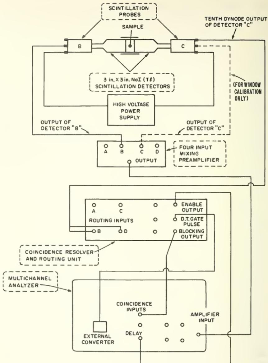
Figure 15. Gamma-gamma coincidence spectrometer.
