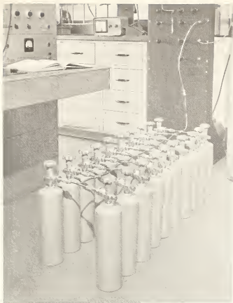
Figure 4. Filling twenty small cylinders from master mixture.
