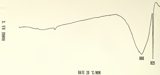
Figure 15. Typical DTA curve for strontium carbonate.
