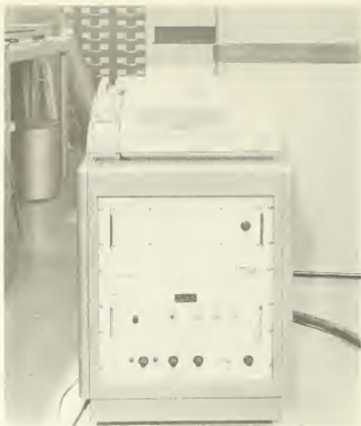
Figure 3. Digital readout for use with emission and x-ray spectrometers.
