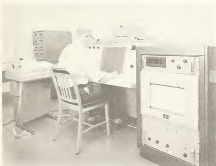
Figure 4. Microphotometer equipped with digital readout for direct entry of data into a computer.
