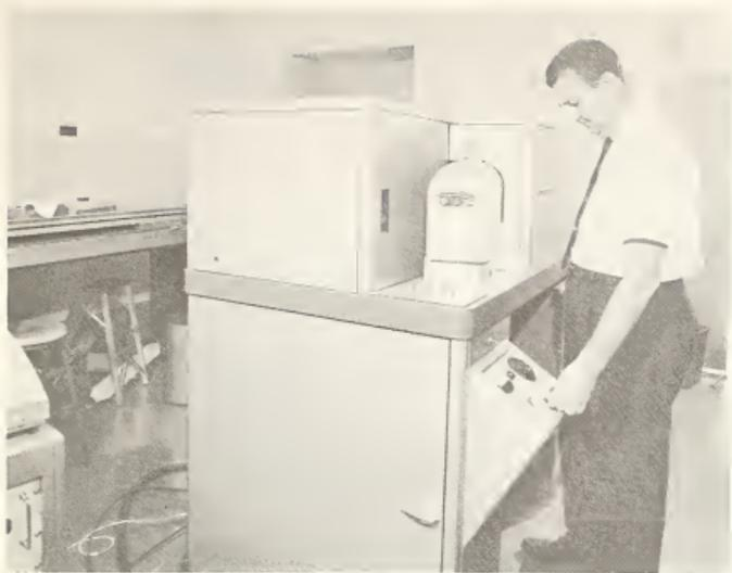
Figure 2. Vacuum spectrometer for the determination of C, P, S, As, Sn and Se in ferrous metals and alloys.
