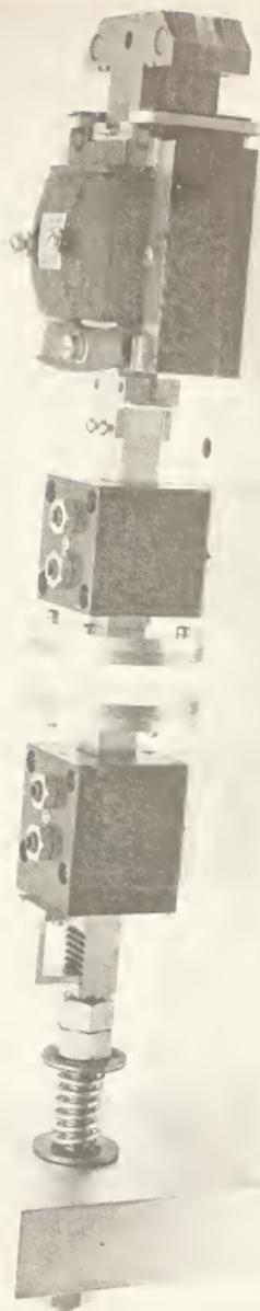
Figure 12. Photograph of the device for rapid quenching of standard reference alloys.
