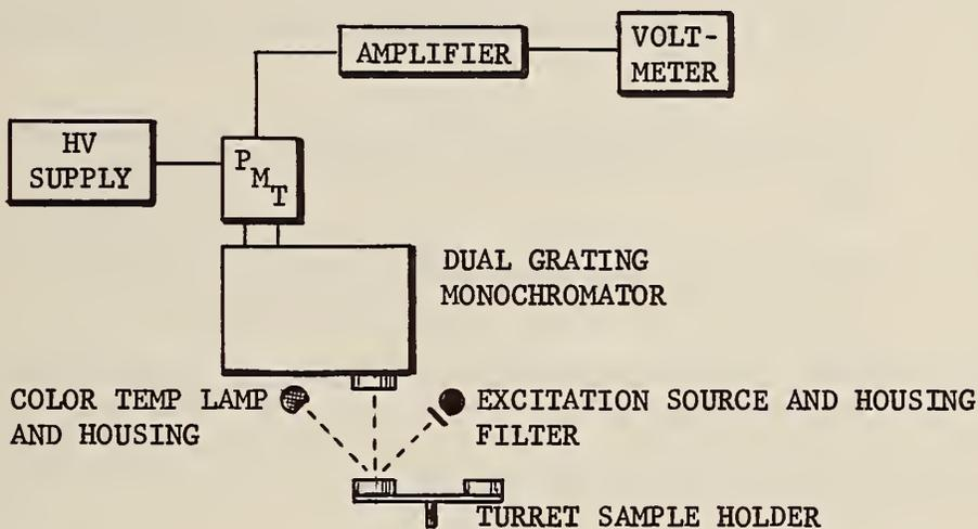
Figure 1 Spectral Measurement Equipment
