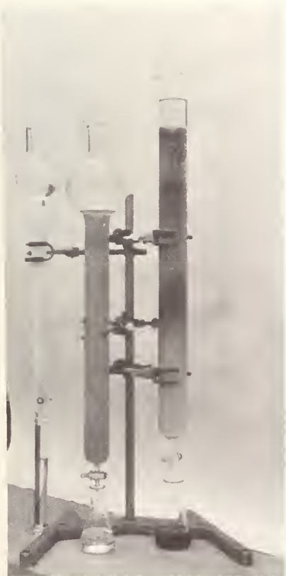
Figure 2. Column separation of oxidation products of pyrene.
