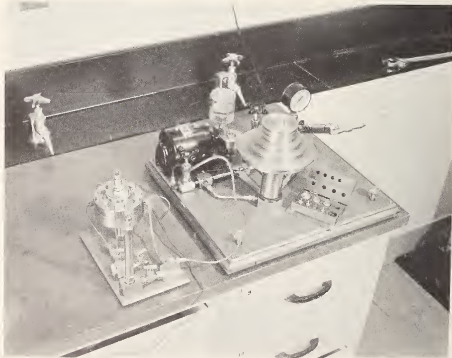
Figure 2. Dead-weight piston gage.
