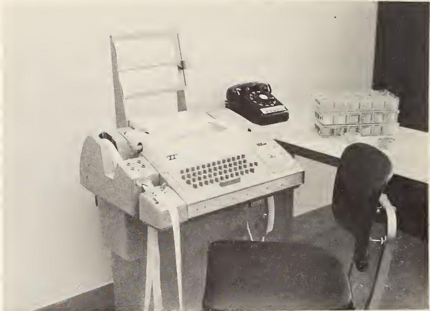
Figure 4. Teletype terminal for communication with time-sharing computer.
