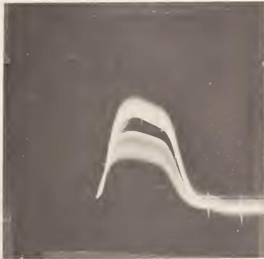
Figure 16. Oscilloscope representation of the amplified pulse output of a gas proportional detector. The pulse height region accepted by the pulse height analyzer, operating in differential mode with a narrow window, is represented by the black wedge.
