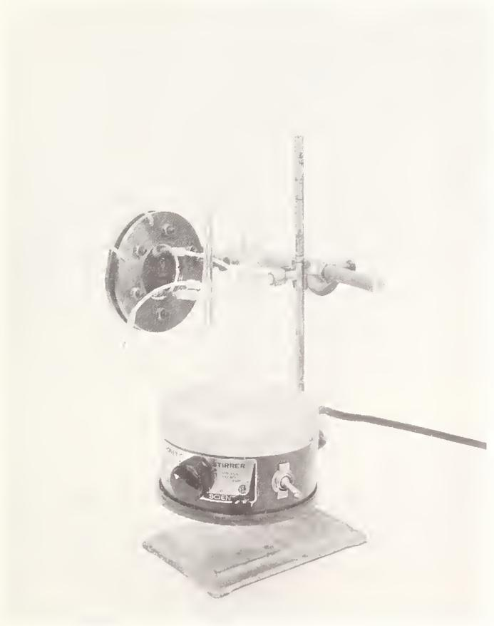
Figure 10. Conductance cell and circulation system for the determination of traces of water.
