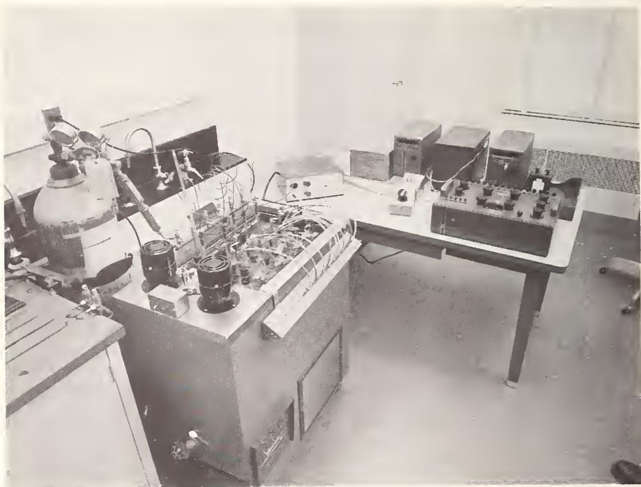
Figure 1. Equipment for the emf measurements on which pH standards in aqueous solution are based.
