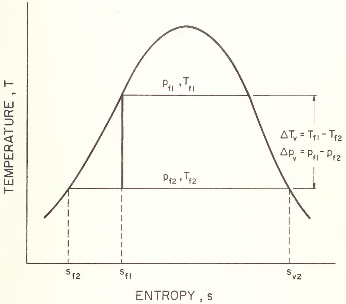
Figure 1. Typical isentropic vaporization process with appropriate nomenclature.
