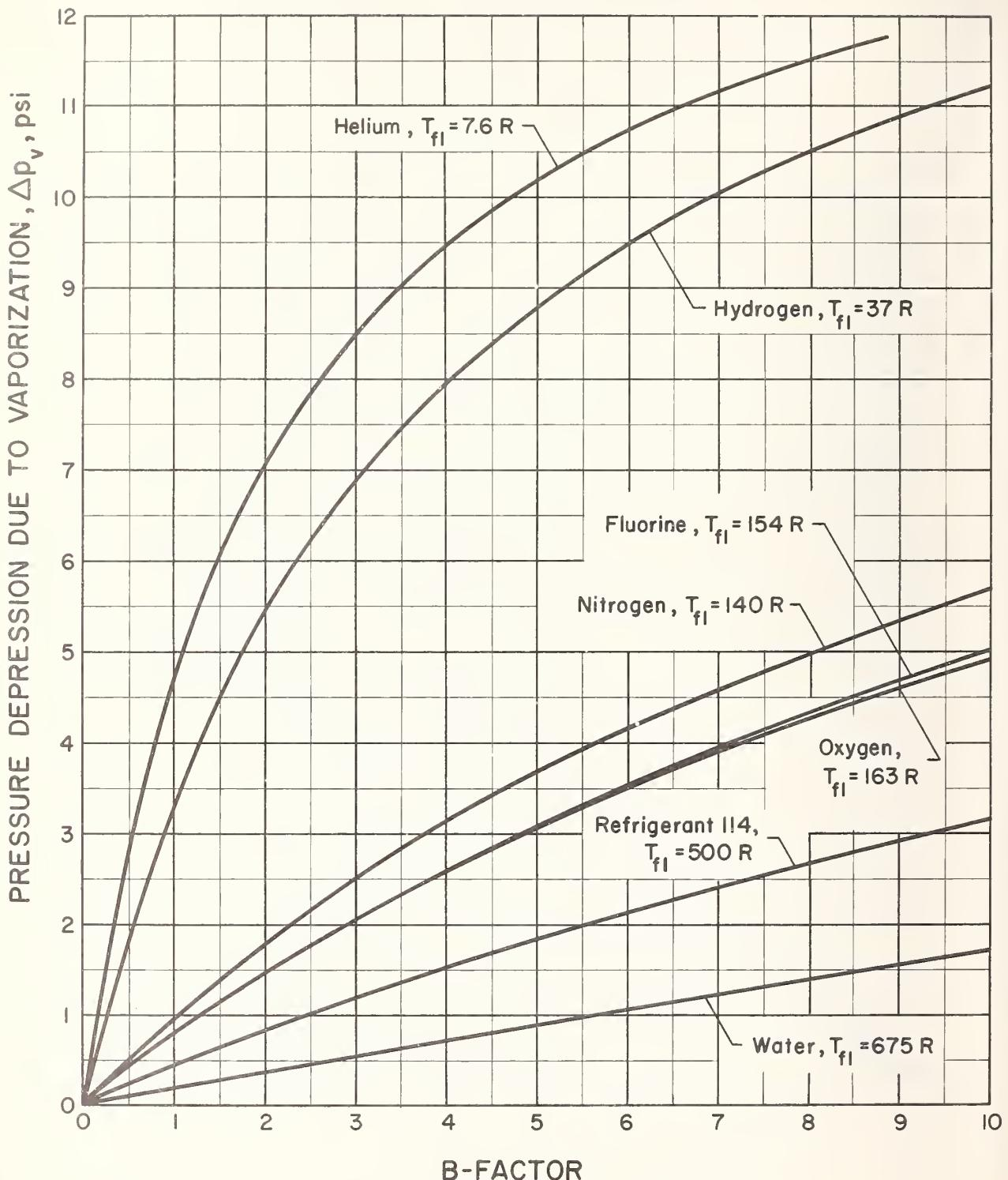
Figure 4b. B-factor and corresponding pressure depressions resulting from isentropic vaporization of various liquids.
