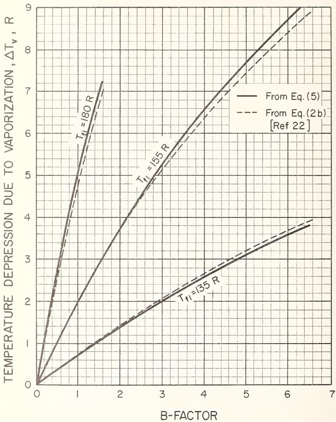
Figure 3. B-factor and corresponding temperature depressions resulting from vaporization of liquid nitrogen.
